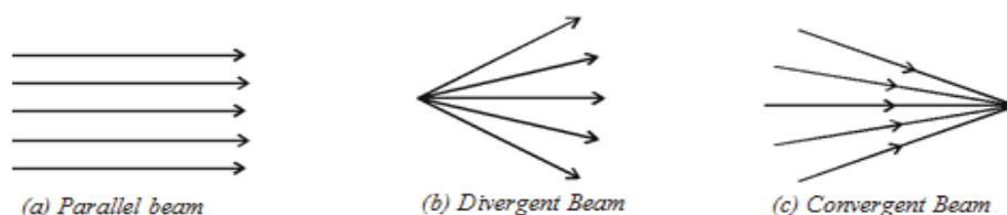
**Fig. 8.1: Beams of light**
