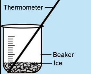
**Fig. 5.4: Determining the lower fixed point on a thermometer**
