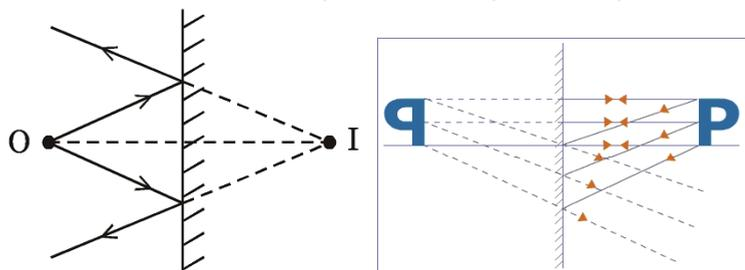
**Fig. 8.9: Image formation in a plane mirror**
