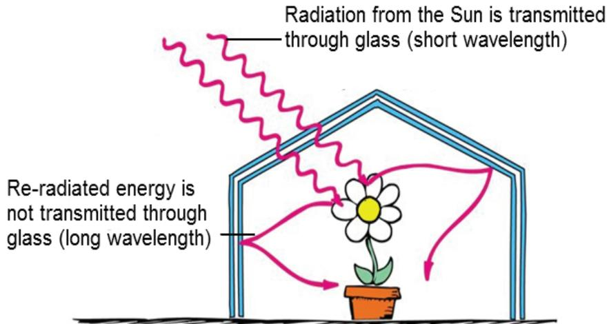
**Fig. 6.21: How radiation keeps a greenhouse warm**
