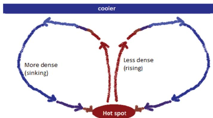
**Fig. 6.7: Illustration of convection**
