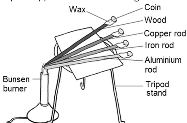
**Fig. 6.5: Investigating rates of conduction**
