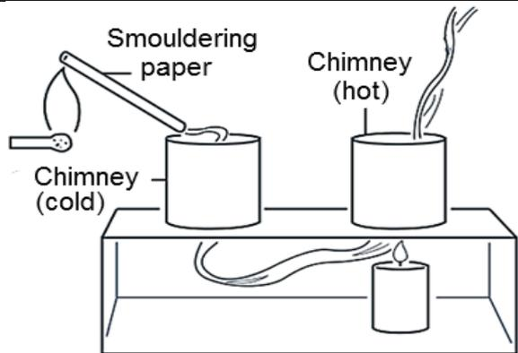
**Fig. 6.10: Demonstrating convection in air**
