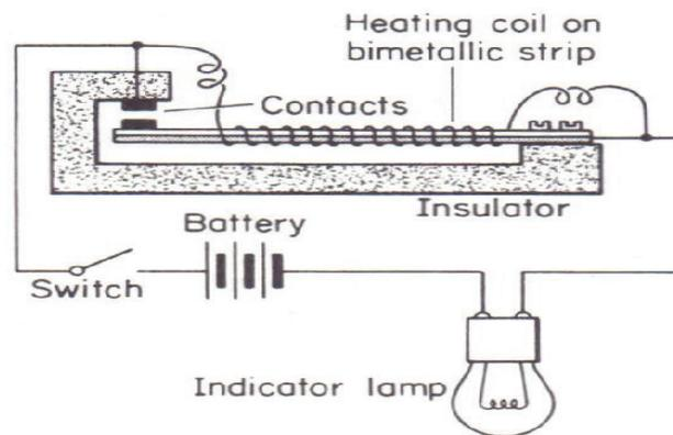
**Fig. 7.3: A flasher unit that uses a thermostat**
