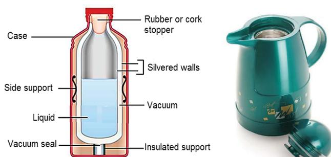
**Fig. 6.20: Parts of a vacuum flask**
