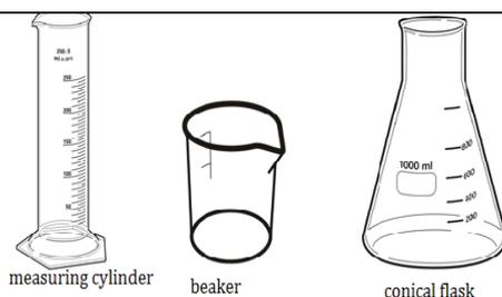
**Fig. 2.11: Apparatus for measuring volume of liquids**
