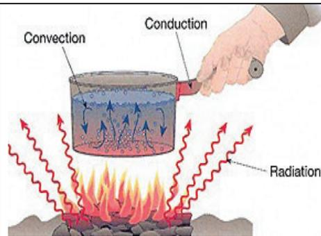
**Fig. 6.2: Processes of heat transfer**
