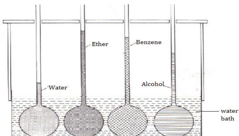
*Fig. 7.6: Comparing liquid expansion*
