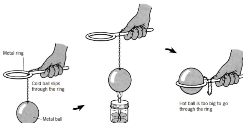
**Fig. 7.1: Ball and ring experiment**
