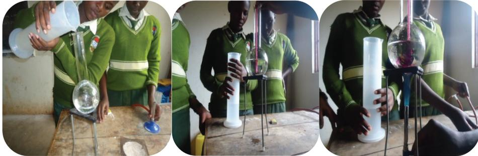
**Fig. 6.9: Demonstration of convection in a liquid**
