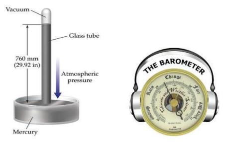
Figure 6.5: A mercury barometer Figure 6.6: An aneroid barometer
